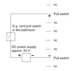
Connection length up to max. 50 meters within the apartment.
