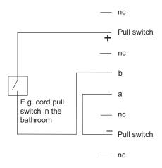
The telephone connection a/b has to supply sufficient power. Pay attention to the polarity of a/b. Pin "a" must be "minus". Connection length approximately 10 - 20 meters within the apartment.
