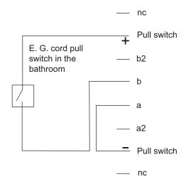
The telephone connection a/b has to supply sufficient power. Pay attention to the polarity of a/b. Pin "a" must be "minus". Connection length approximately 10 - 20 meters within the apartment.
