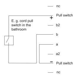
The telephone connection a/b has to supply sufficient power. Pay attention to the polarity of a/b. Pin "a" must be "minus". Connection length approximately 10 - 20 meters within the apartment.
