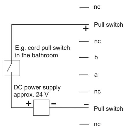
Connection length up to max. 50 meters within the apartment.
