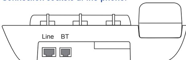
„Line“ socket: Connection of a/b and cord pull switches (contact input). „BT“ socket: Connection of a pear switch.
